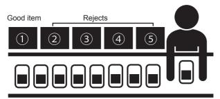
Products are sorted into good items and defective ones and inputted. The defective products are sorted into each cause. The timestamp and the number of occurrence times are recorded when defective products occurred.
