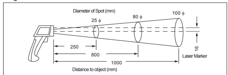
Above diagram shows the Field of View (Spot Size) increases when distance from the sensor tip to the object increases.
